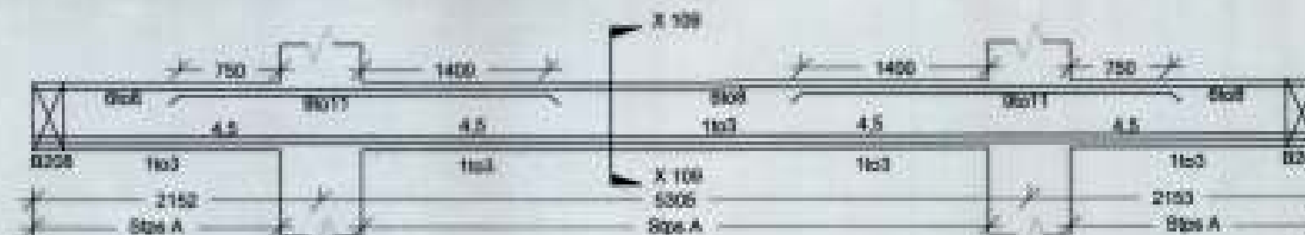
B-109 Bars: 1 to 11 =16mm dia. Stps A; 8mm dia.2L 9 Nos. @ 100mm c/c & rest @ 200mm c/c
