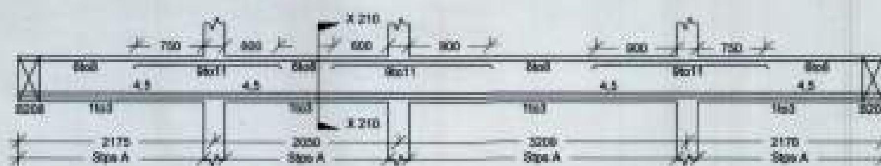
B-210 Bars: 1 to 11 = 16mm dia. Stps A: 8mm dia. 2L 9 Nos. @ 100mm c/c & rest @ 200mm c/c
