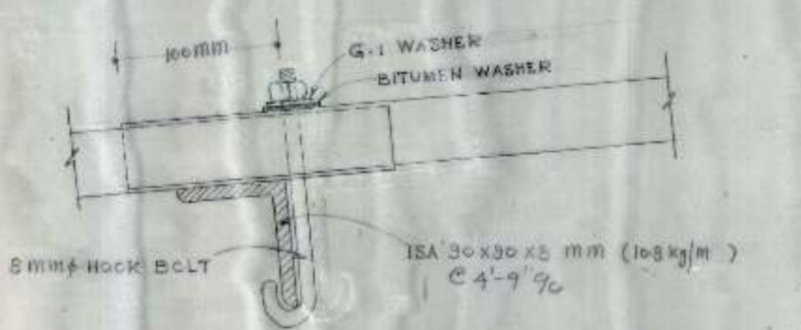
CONNECTION OF PURLIN WITH A.C. SHEET
